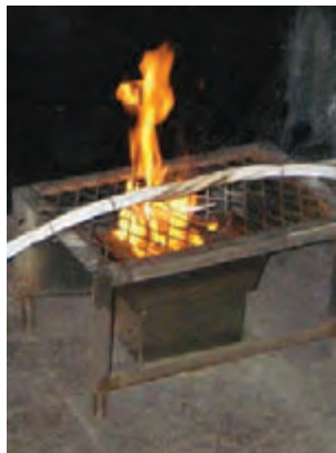
3m 3 smoke test to IEC 61034
